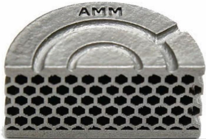
are possible. AM will yield far less part mass with reduction factors of three or four times those of other technologies. This is because we can grow much thinner-wall structures and supports that would be difficult or impossible, and far more expensive, in subtractive technologies. Also, this work is performed without tooling or casting expenditures.
