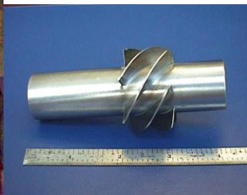
IN 625 LC Propeller blades on shaft
